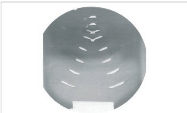
Fig. 4 – Picture series of schlieren photos of the cylinder shock wave: schlieren photograph of the fronts of successive waves on the way from the reflector to the treatment zone.
