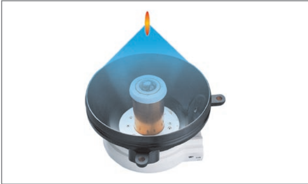
Fig. 3 – Cylindrical source with parabolic reflector: a coil is wound around a hollow cylinder and covered with an insulating layer and a conductive membrane. An electric shock generates repellent electromagnetic forces that radiate a cylindrical pressure wave at right angles to the cylinder axis, according to the geometry of the arrangement. The wave is transformed into a convergent spherical wave through reflection on the paraboloid reflector and is concentrated in the treatment zone.
