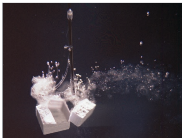
Fig. 14 – Stones with separation of fragments: effect of a focused shock wave on a cube-shaped artificial stone with an edge length of 10 mm (shock wave occurrence from the right). One can see the stone held on a wire, the fragmentation into a few concretions and cavitation bubbles in the shock wave path.
